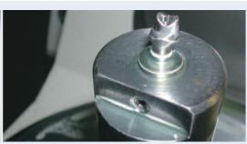
Fig. 9 Laboratory image of the definitive Encode Abutment just prior to removal from the milling unit.
